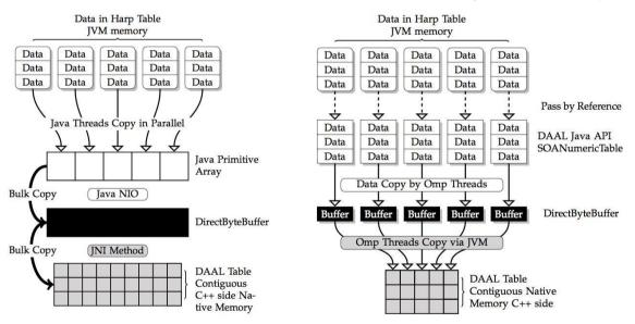
Figure 2. Direct Bulk Copy (left) vs. Multi-threading irregular Copy (right)
