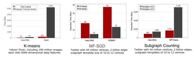
Figure 3. Performance Comparison on three different important machine learning algorithms: Kmeans, MF-SGD and Subgraph counting.
